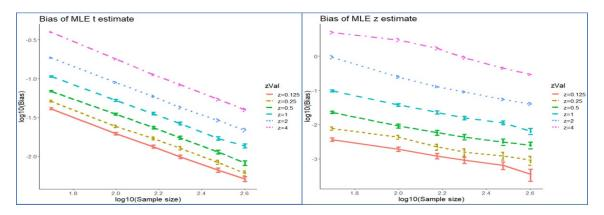
Figure 2: Log-log plots of empirical biases for MLE estimates of t and z as a function of sample size. Different curves are for different actual values of z for the sampled distribution (indicated by 'zVal' in the legend), while the actual value of t was 1 for all cases. Error bars show plus or minus two standard deviations in the bias estimates.
